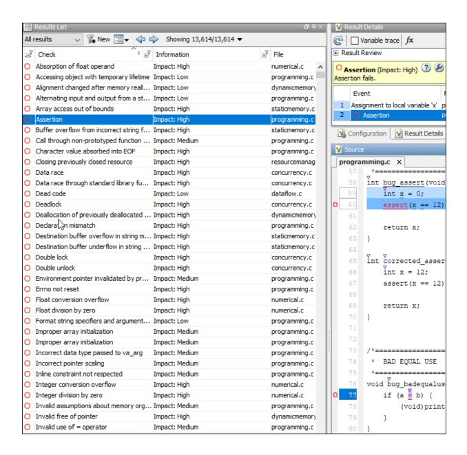
**Benefits:** To find the root cause of a result, you have to navigate through the source code. You can keep the result pinned on the **Results List** and **Result Details** pane during this navigation.
